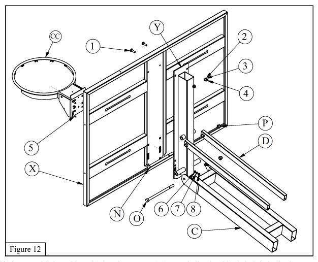
14. Lift the assembled *Backboard* (X) and *H-Frame* (Y) up and align it with the bolt holes in the *Lower Arm* (C). Using a 5/8" X 12" Hex Bolt (O) and 5/8" Lock Nut (P) attach the Backboard (X) to the Lower Arm (C). Tilt the Backboard (X) up and attach it to the Upper Arms (D) with a 5/8" X 11" Hex Bolt (N) and 5/8" Lock Nut (P). Tighten and then back off 1/2 turn. See Figure 13
