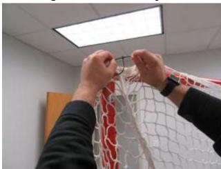
9. Using (1) NET TIE, connect rear of NET to back of V-SHAPED GROUND BAR CONNECTOR as shown.
