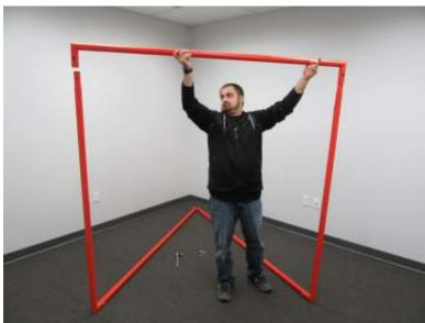
6. With head of  $3/8" \times 2"$  HEX BOLT seated into slot on front of HEADER BAR, connect each side of HEADER BAR to UPRIGHTS using (1)  $3/8" \times 2"$  HEX BOLT, (1) FLAT WASHER and (1) LOCK NUT as shown below.
