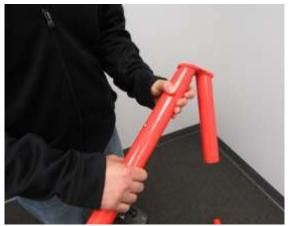
2. Connect (1) SPLICE CONNECTOR to the opposite end of both GROUND BARS as shown below.
