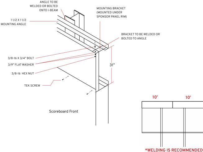
HARDWARE FOR BOLTING SUPPLIED BY INSTALLER
