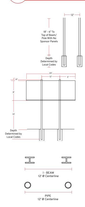
The following information for installing the mounting poles/ beams are suggestions only. Local codes, field placement, scoreboard options, customer preference, and other special considerations will determine the specifics of your installation, including footer specifications, above ground height, and total length of the poles/I-beams.
