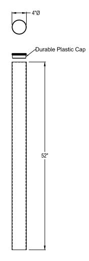
Ground sleeves shall be constructed out of a 4" outside diameter steel tube with a galvanized finish and have an interior diameter of 3 19/25". Product is 52" long providing for depth in a sand volleyball court and proper drainage. A durable plastic cap is provided to keep sand out. Installation to be completed in accordance to manufacturer's instructions. Do not scale drawings. Each sleeve shall weigh approximately 35#.
